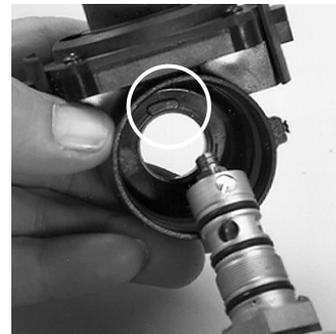
**Note:** Resistance will develop when the O-ring is forced into its seat. The valve core is seated when it will not rotate.
